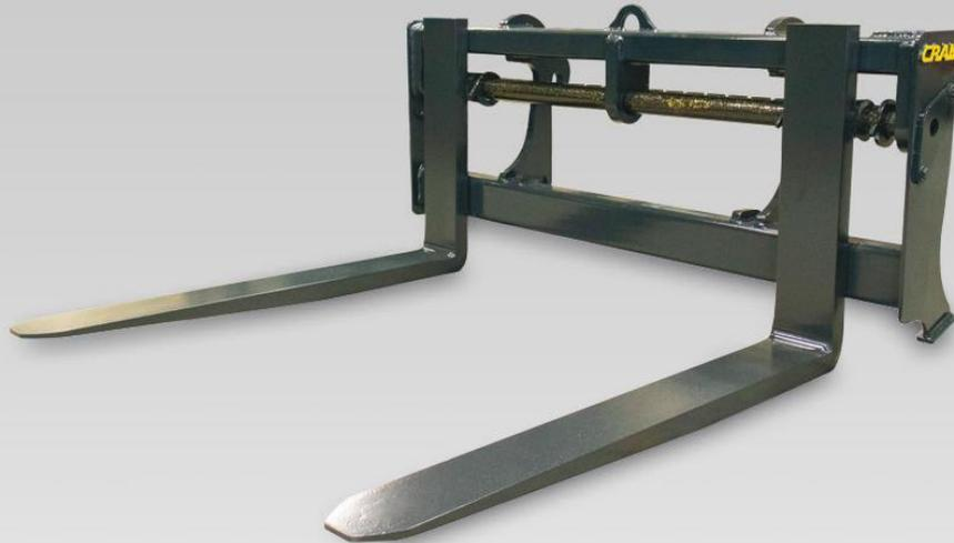
Designed for smaller machines, this version of our Pallet Forks features adjustable tines on a single hanger bar. The tine hanger bar features tine locks to keep tines in place once positioned. A low profile, simplified back frame design allows maximum visibility to the tines for added job site safety.
